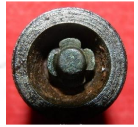
Percussion cap installed on nipple
